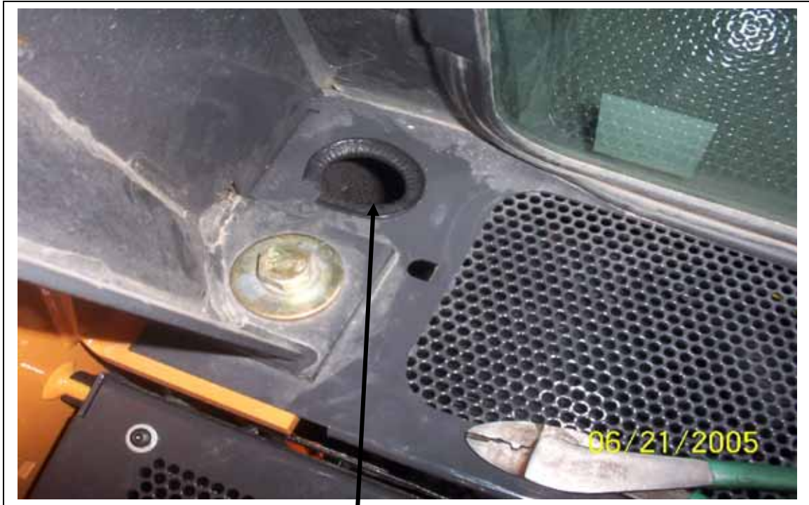
Knock out at left side behind rear window. Install trim as shown.
