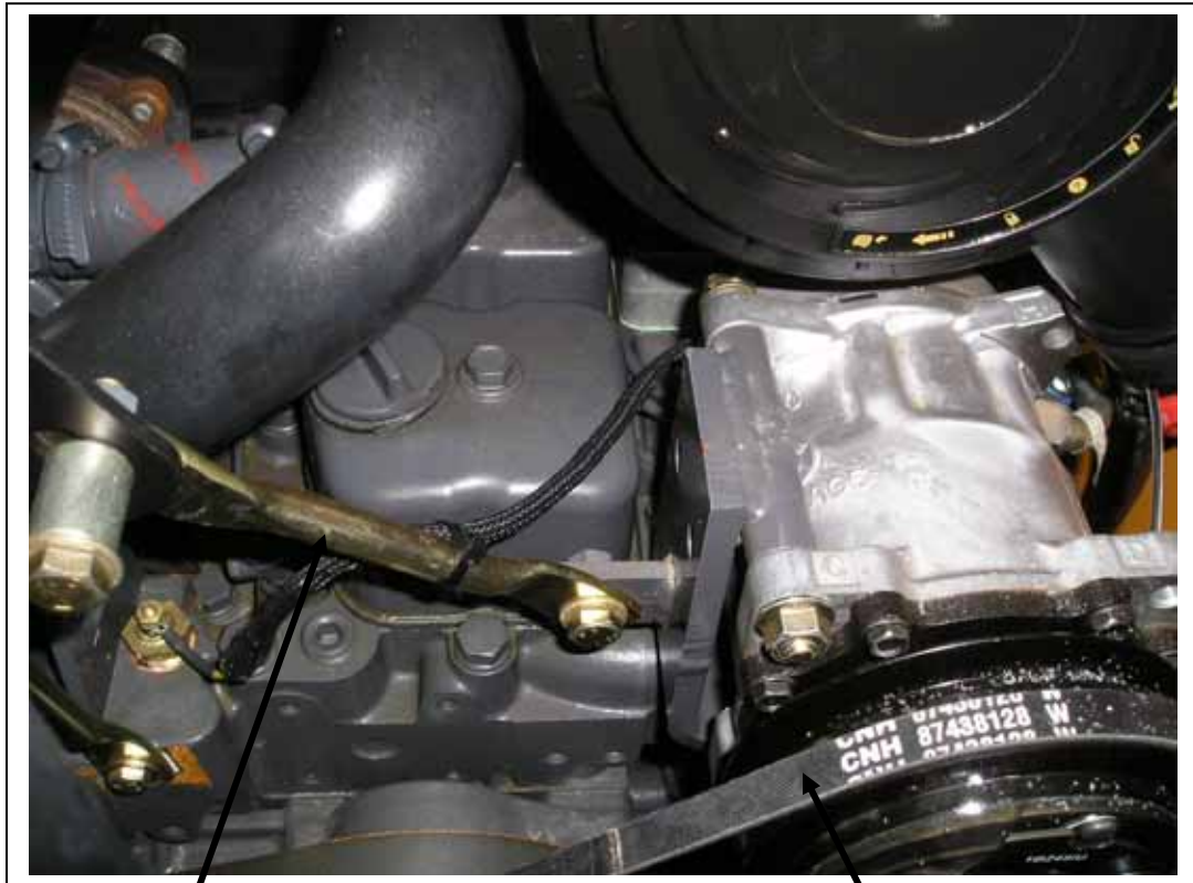
Compressor mount stiffener bracket.
